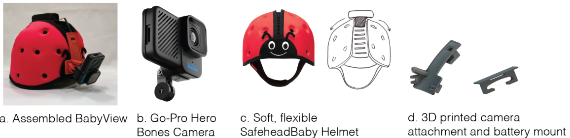
Figure 2. Overview of the BabyView Camera design process, showing (a) the assembled device, (b) the original camera, (c) babysafe helmet, and (d) and 3D printed mounting equipment.
