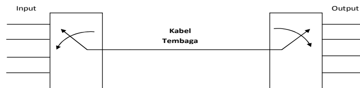
Fig. 5. Block Diagram of the Analog Signal Measurement TDM with Conductor Cable
