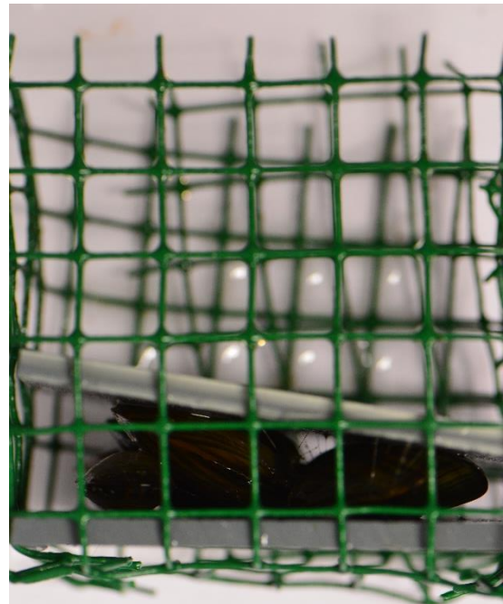
Figure 15; Mussels are placed between two PVC plates, surrounded with chicken fence.
