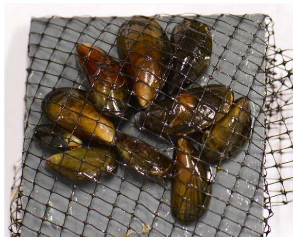
Figure 16; Mussels are kept in place on a PVC plate using a small net. The net is fixed by using a tie-wrap at the back.
