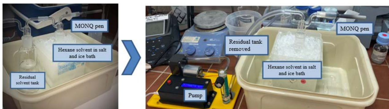
Figure 7 Unsuccessful vapour analysis set ups. Dual impingers (right) were replaced with a direct connection to the auto pump (left) to see if this provided any results.
