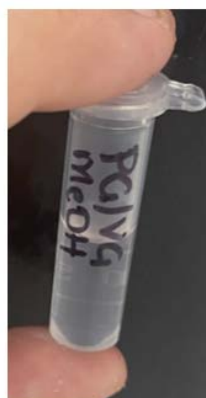
Figure 9 Miscibility tests showing that PG/VG is miscible in DCM and MeOH but not in Hexane.
