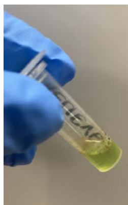
Figure 8 Photo showing separation between carrier fluid and essential oil in MONQ Relieve after standing on the bench at room temperature for several days
