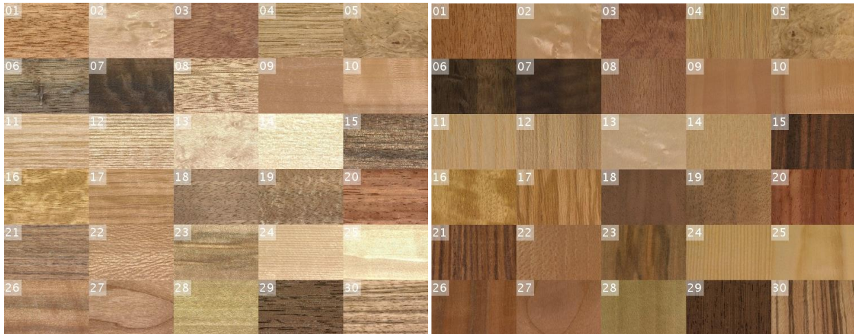
Fig. 1. All 30 samples of wood veneer for (left) specular, (right) non-specular (90 degree rotated) view/light geometries.
