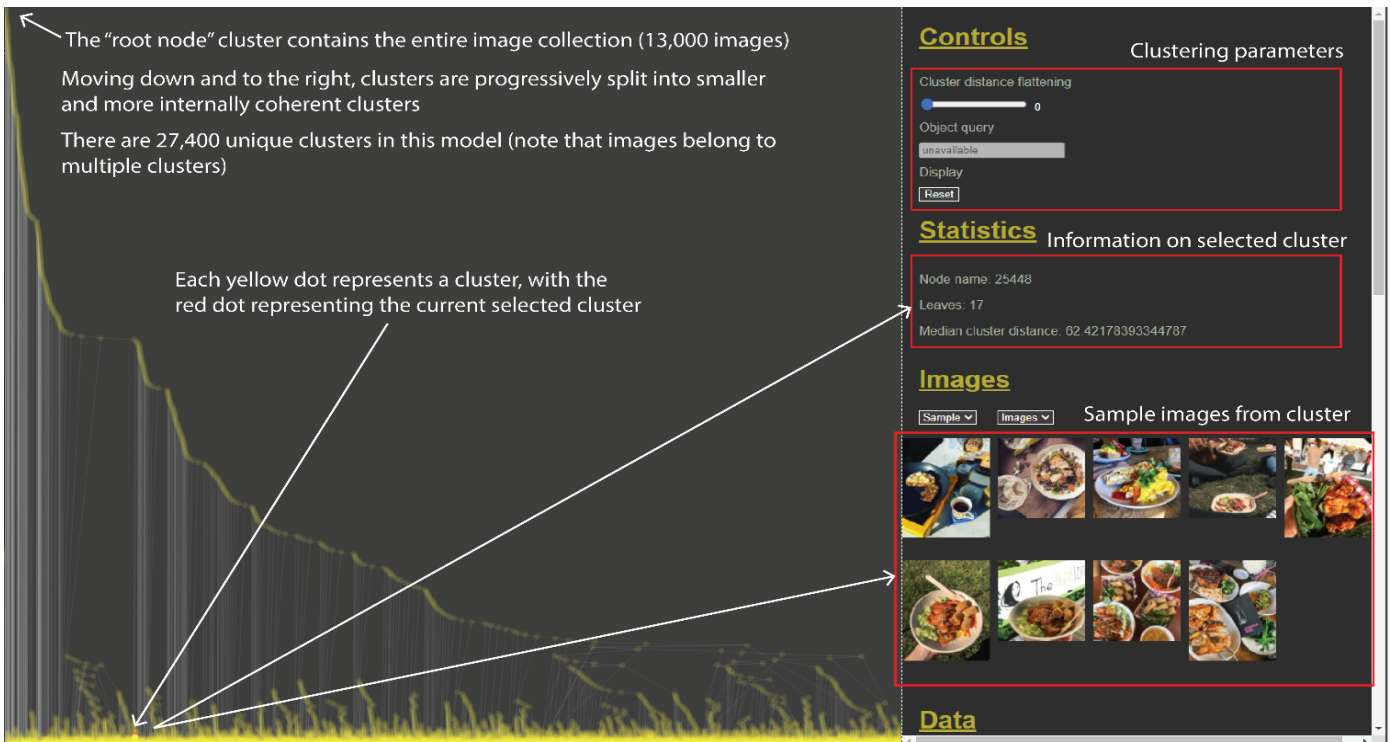
Figure 2. The visualisation module allows clustered image data to be visualised and interrogated. In this example the VGG16 embedding is combined with a hierarchical clustering, operating over a corpus of images from Instagram.
